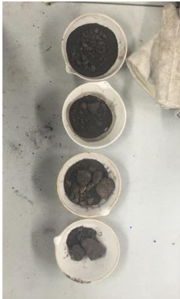
Caption- These are soil samples collected in the field and analyzed in the Geotechnical Engineering Lab. These samples were mashed up in order to determine the sieve analysis and soil classification.
