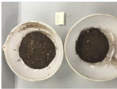
Caption- These are soil samples that were collected out in the field and analyzed in the Geotechnical Engineering Lab. These samples are mostly made up of a silt clay-like material with some rock present.
