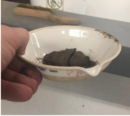
Caption-This is a soil sample that Ryan King just took out of the oven and is ready to determine the soil's moisture content.
