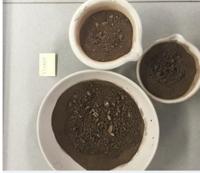
Caption- These are soil samples that were collected out in the field and analyzed in the Geotechnical Engineering Lab. These samples are mostly made of a silt material with a small trace of rock.
