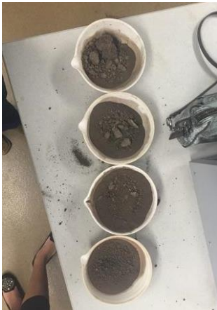
Caption-These are soil samples that Hasan Mohammad and Leah Richardson are getting ready to mash up for the sieve analysis and soil classification.
