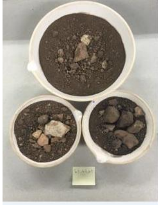
Caption- These are soil samples collected in the field and analyzed in the Geotechnical Engineering Lab. These samples appear to have some type of sandy clay and large amounts of rock present in them.
