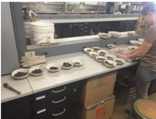
Caption-These are soil samples that Holly Swenson is mashing up for the sieve analysis and soil classification.
