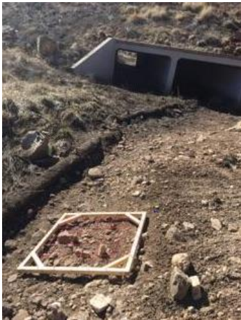
Caption- This is a part of Sinclair Wash Trail where the rock grid was used in order to do the pebble count.
